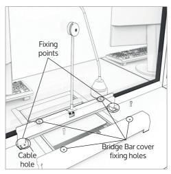
5. Feed wiring through the cable hole back to the amplifier. Using provided fixing holes and screws, attach the bridge bar cover carefully to avoid damage to wiring.
