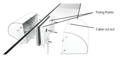
7. Install the power supply close to a power socket outlet using the supplied mounting bracket and fixing screws.
